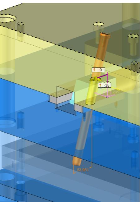
• Adjust the **measured stroke** to 49.9mm.
