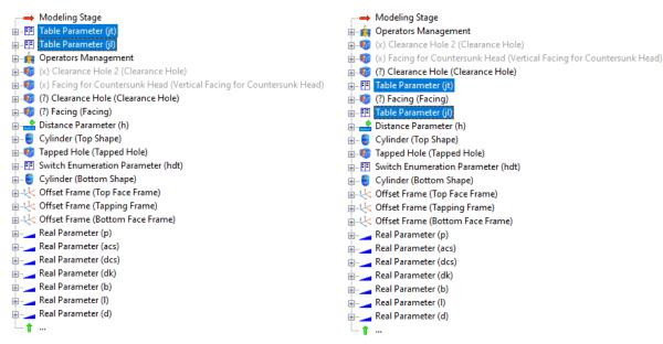
• Always from the Operations tree, edit the **Facing** operation and replace the screw spot facing operation by a flat-bottomed blind hole with a diameter equal to *dk+jl* and a depth equal to *h*.
