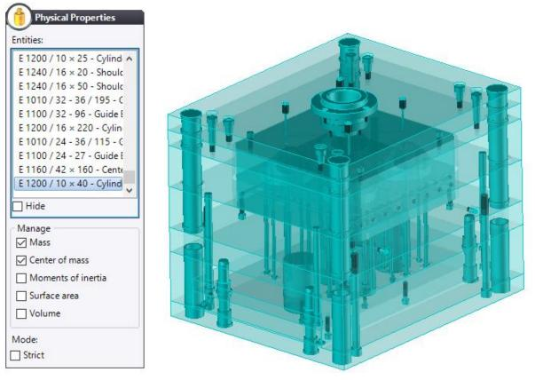
If you want to position a lifting eye bolt on the A side and B side, you have to select the parts of the B side set, and then select those of the A side set. You will then have three centers of mass: one for the whole mold and two for the fixed and movable parts of the mold.
