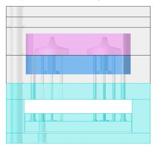
• For the third screw, drag and drop the **E 1200** component to fix the core block and the B plate. Enter the following values for the dimensioning and positioning.
