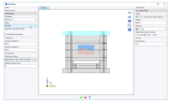
The parameters on the right of the dialog box are the parameters for a plate of the mold base. You can select the plate from the **Component** drop-down list.
