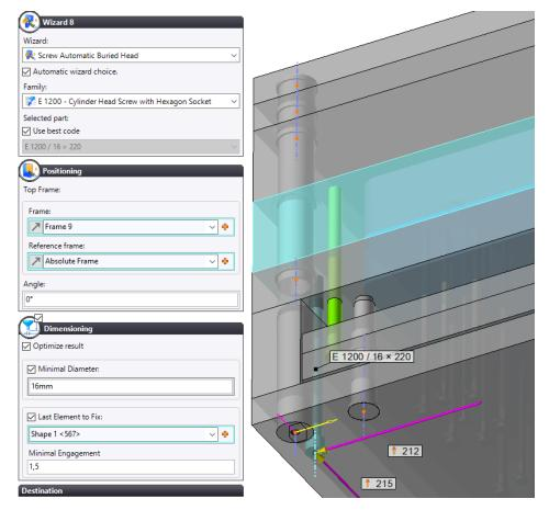
After confirming the wizard, the process dialog box appears. Various processes are possible for this type of component.
