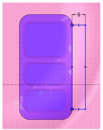
• Create a second sketch as shown below on the same top face of the cavity block's rectangular insert, then **confirm** the sketch. This sketch represents the shape of the process.
