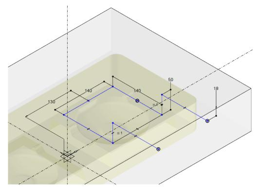
• To define the exit, right-click on the segment or cylinder of the exit drilling and select the T Set As Exit command.
