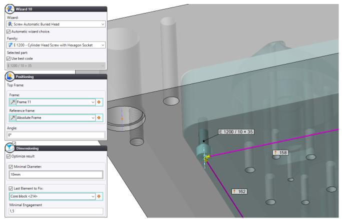
• After confirming the wizard, select the **Tapped hole** process in the **Use Process** dialog box.
