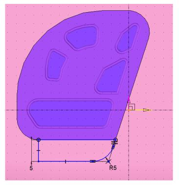
• Create a second sketch as shown below on the same top face of the cavity block's center insert, then **confirm** the sketch. This sketch represents the shape of the process.
