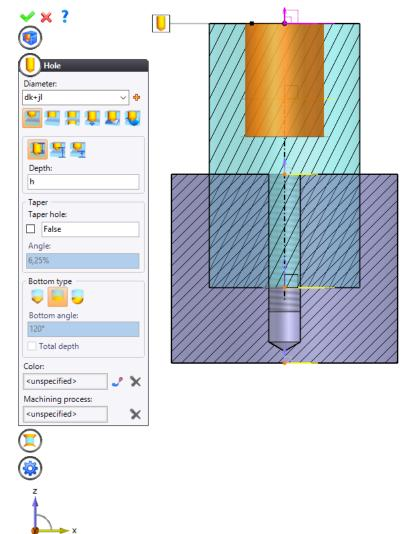
• Edit the **Clearance Hole** operation and replace the clearance hole operation by a blind hole with a diameter equal to *d*+*jt* and a depth equal to *l*.
