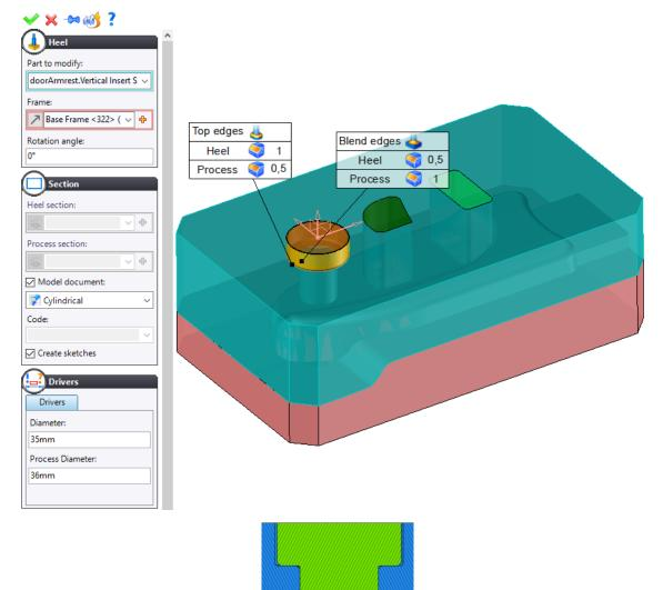
**Note**: You can create the sketches on the fly or select existing profiles for the heel and process sections using the special inputs.
