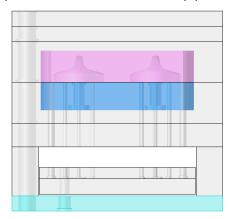
• For the second screw, drag and drop the **E 1200** component into the graphics area to fix the ejector retaining plate and the ejector base plate. Enter the following values for the dimensioning and positioning.
