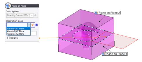
The absolute frame will represent the mold zero point. It is located this way because we will subsequently repeat the core and cavity blocks to make a total of four.
