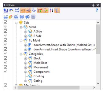
They are also available in the Parts tree. As well as being able to view the sets and parts, you can also filter the elements by **function** (plate, ejector base plate, guide pin, screw, inserts, etc.).
