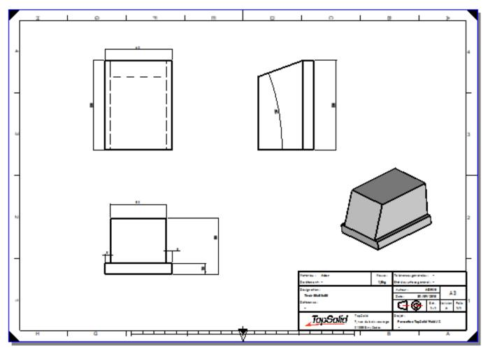
In order to save time when setting the dimensions, display the annotations of the front view. To do this, rightclick on the front view and select the **Projected Annotations** command.
