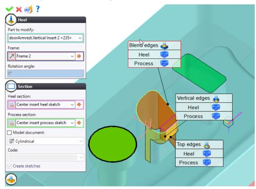
• Create a **heel** on the last insert of the cavity block using a rectangular profile. Select **None** for the **top**, **vertical** and **blend edges**.
