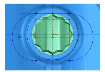
• From the **Mold** tab, select the 4 **Heel** command and adjust the parameters as indicated below.
