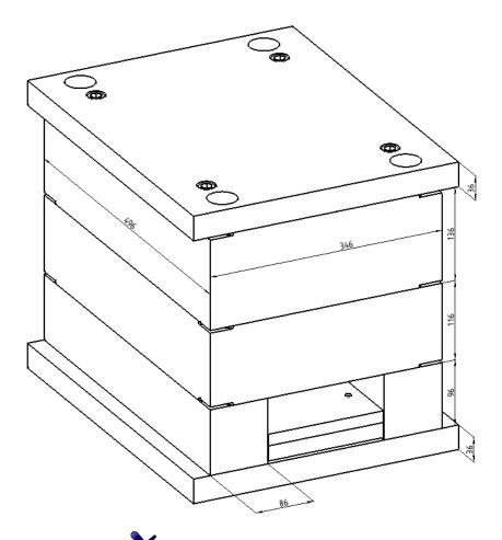
• From the Assembly tab, select the **X** Removing command and select the two core and cavity blocks.
