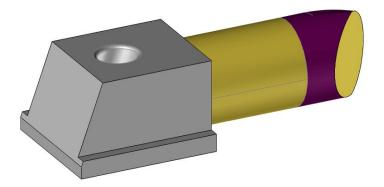
Because of the union between the insert and the slide, there is an extra part in the assembly. To avoid this, you can delete the insert as an operation.
