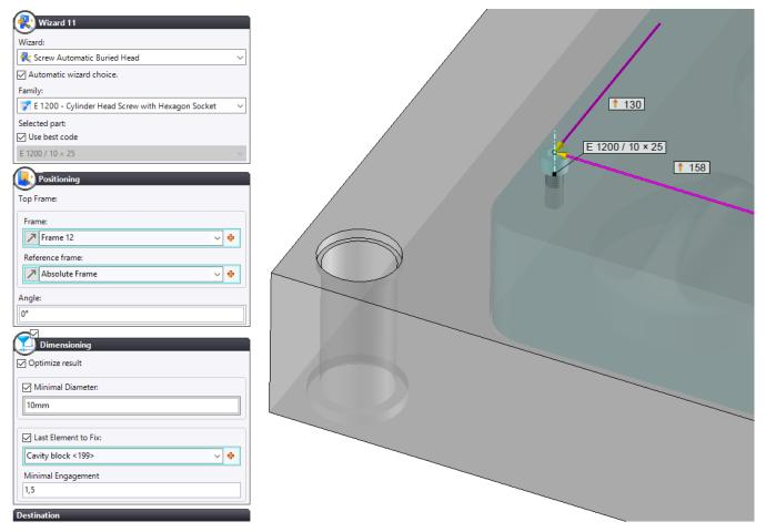
• After confirming the wizard, select the **Tapped hole** process in the **Use Process** dialog box.
