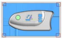
• Hide the mold base. To do this, click on the **Hide/Show Mold Base** icon at the bottom right of the graphics area.
