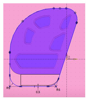
• Create a new sketch as shown below on the top face of the cavity block's rectangular insert, then **confirm** the sketch. This sketch represents the shape of the heel.
