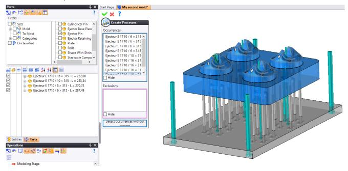
• From the Operations tree, select all the pin processes and create a folder named *Pin processes*.
