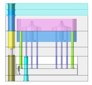
• For the fourth screw, drag and drop the **E 1200** component into the graphics area to fix the cavity block and the A plate. Enter the following values for the dimensioning and positioning.
