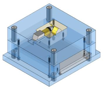
**Note**: If necessary, you can modify the slide process by editing it from the Operations tree. You can modify the process length for large molds (by default 500mm).
